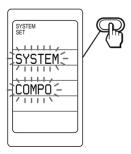
The macro numbers are displayed on the labels. To change the labels (SONY OFF, SYSTEM2-12), press the SCROLL button repeatedly. The macro numbers for which the system macro is programmed stay lit, and others flash.
